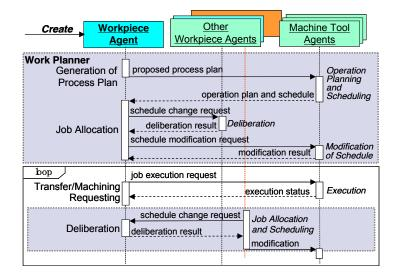
Figure 4. Sequence flow for the machining process
