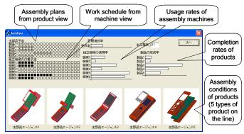
Figure 7. Display of the assembly simulation
