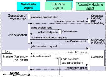
Figure 5. Sequence flow for the assembly process
