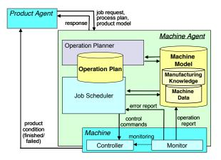
*Figure 3*. Structure of the machine agent
