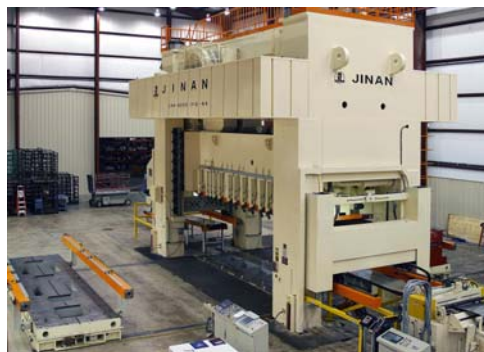
Figure 1 – Mechanical press's pre-assembly in factory
