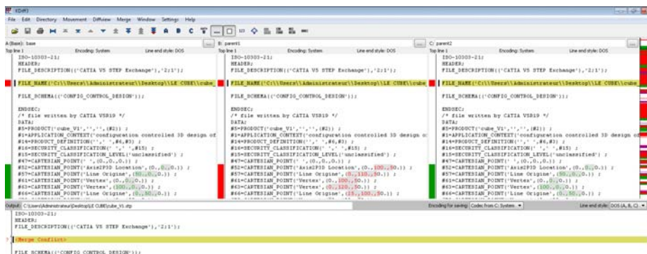
Fig. 8. Classical 3-way merge tool used on STEP files
