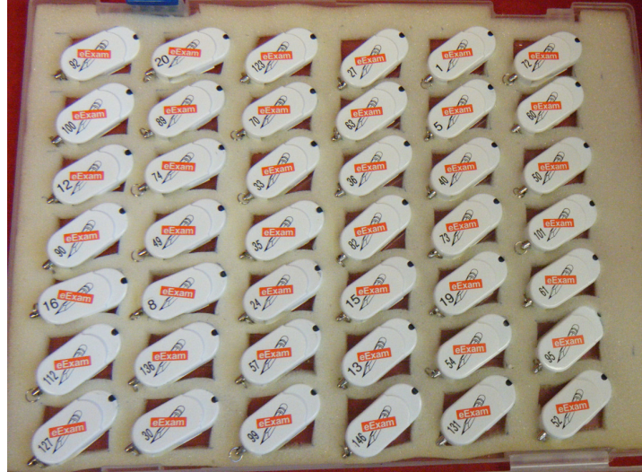
Fig. 1. A set of USB sticks each containing the eExamination system, question paper and answer partition
