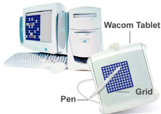
Figure 4. AudioBattleShip input device for blind players [18]
