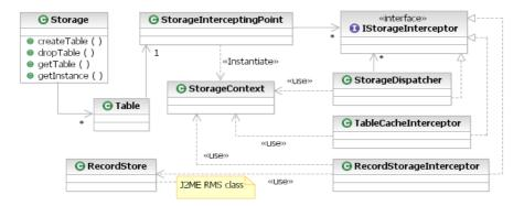
**Fig. 2.** Simplified class diagram depicting interceptor design pattern involvement in architecture and how the custom interceptors can be passed from Storage initialization through Table to StorageInterceptingPoint class.
