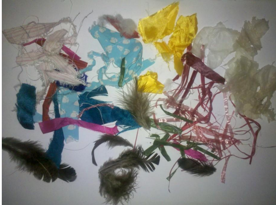
Fig. 1 Foreign fiber samples.
