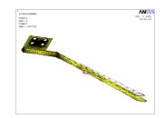
Fig.7 Distribution nephogram of roller tooth bearing force
