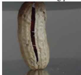
(a) Cracking longitudinally
