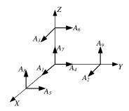
Fig. 2. Nine-accelerometer NGMIMU configuration
