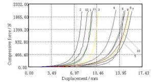
**Fig. 6.** Compression curves of fish floss with different moisture content 1, 2 and 3: compression curves of fish floss with the moisture content of 23.57% 4, 5 and 6: compression curves of fish floss with the moisture content of 19.32% 7, 8 and 9: compression curves of fish floss with the moisture content of 10.39% 10, 11 and 12: compression curves of fish floss with the moisture content of 5.13%
