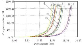
**Fig. 5.** Compression curves of fish floss with different particle sizes 3, 6, 8 and 14: compression curves of fish floss with the drying time of 10s 5, 9, 11 and 13: compression curves of fish floss with the drying time of 20s
