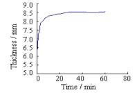
Fig. 2. Relaxation characteristic curve of molding block
