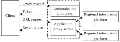
Fig. 3. SSO system architecture
