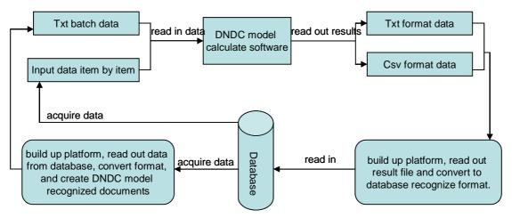
Fig2. Main functions logic diagram of assistant DNDC module
