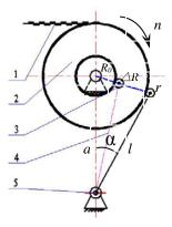
1 seed tape; 2 seed tape disk; 3 seed tape disk radius detection roller; 4 seed tape disk radius detecting pendulum; 5 angular displacement sensor
