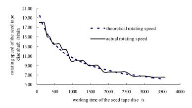
Fig. 4. Contrast curves of theoretical and actual rotating speed of the seed tape disk
