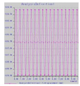
Fig.6 Vertical displacement of the bottom shovel tip
