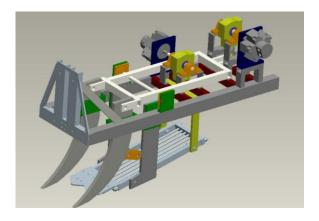
Fig.2 The digital element model of the 1WZ-type deep rhizome crops excavating test-bed
