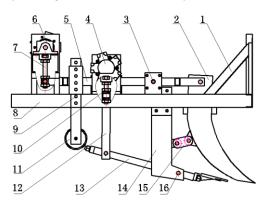
Fig.1 The structure of the 1WZ- type deep rhizome crops excavating test-bed
