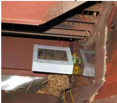
Fig.8: sensor's installation position
