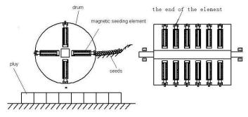
Figure 1. schematic diagram of Precision Seeder
