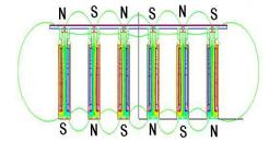
Figure 5.NN order of space distribution of magnetic field lines of magnetic force
