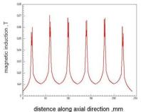
Figure 7. the curve of magnetic induction intensity in the order of NN along the axial direction
