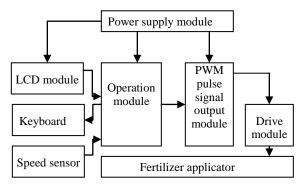
Fig.1 The structure of semi-automatic variable rate
