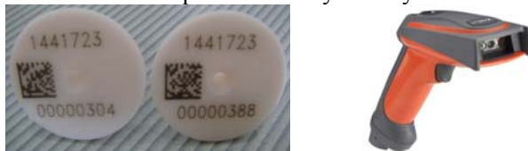
Fig.2 DM-bar ear tag(left) and all purpose bar scanner
