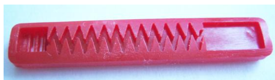
Fig.1: An injection molded emitter with labyrinth channels
