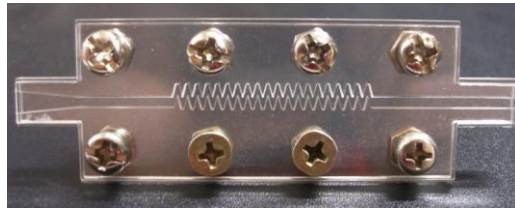
Fig.6: The test model of labyrinth channels fabricated in plexiglass
