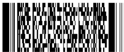
Fig.1: Structure of PDF417
