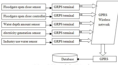
Figure 4. Transmission Network
