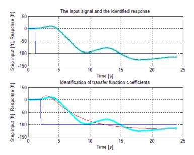
Fig. 5. Pilot's response to a unit step function – descent to the original altitude (oscillation)
