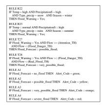
Fig. 5. Rules for flood forecasting from the knowledge base of the INTELLEnvQ system
