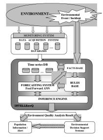
Fig. 3. The architecture of the INTELLEnvQ system
