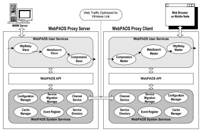
Fig 1. The WebPADS system architecture
