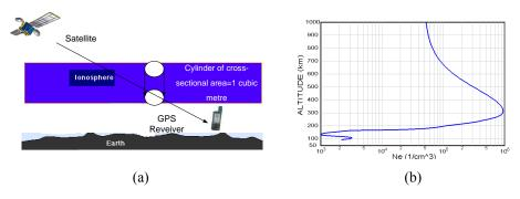
Fig. 1. TEC representation and typical electron density profile of the ionosphere over Cyprus.
