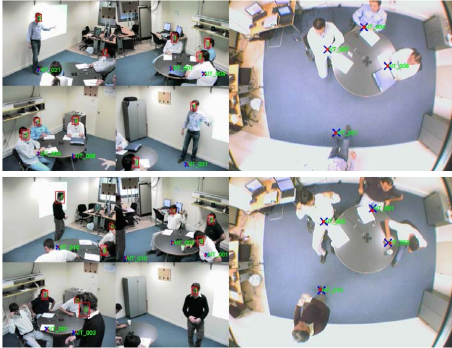
Fig. 2. Operation of the individual 2D face trackers on the four corner cameras and association of the 2D evidence into 3D tracks. The detected faces are marked by bounding boxes. The IDs of the tracks are of the form AIT_XXX shown at the projection of the tracked head centroids on the floor. The tracks are also projected to a panoramic camera (not used by the system) for better visualization
