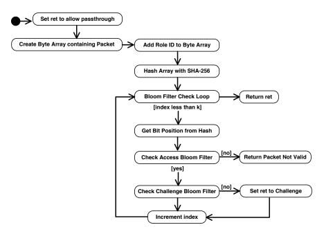
Figure 3. Flow diagram of the access control logic.
