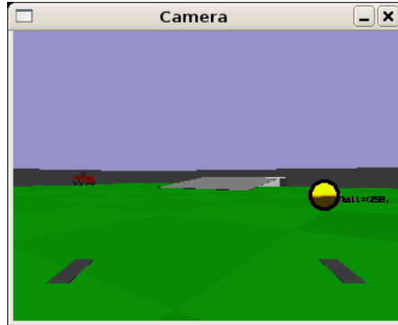
Fig. 3 The perception of the robot that we use in our experiments. It shows one camera image with the ball that has been recognized by our vision algorithm.
