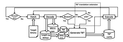
Fig. 4. Modified basic block translation (adapted from [10]).
