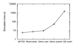
Fig. 5. Simulation overhead increase at different refinement levels.
