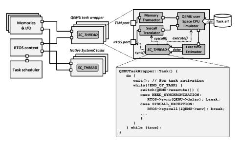
Fig. 2. Mixed level simulation by QEMU task wrapper.
