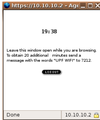
Fig. 4. The pop-up window to keep the connection open. A count-down timer indicates the credit.
