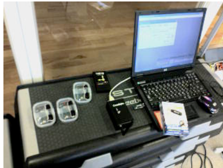
Fig. 5 Sensor Zigbee devices and gateway PC
