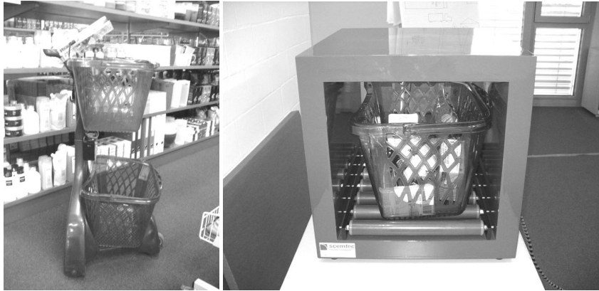
Fig. 1. Shopping trolley and tunnel reader in the Migros Smart Store
