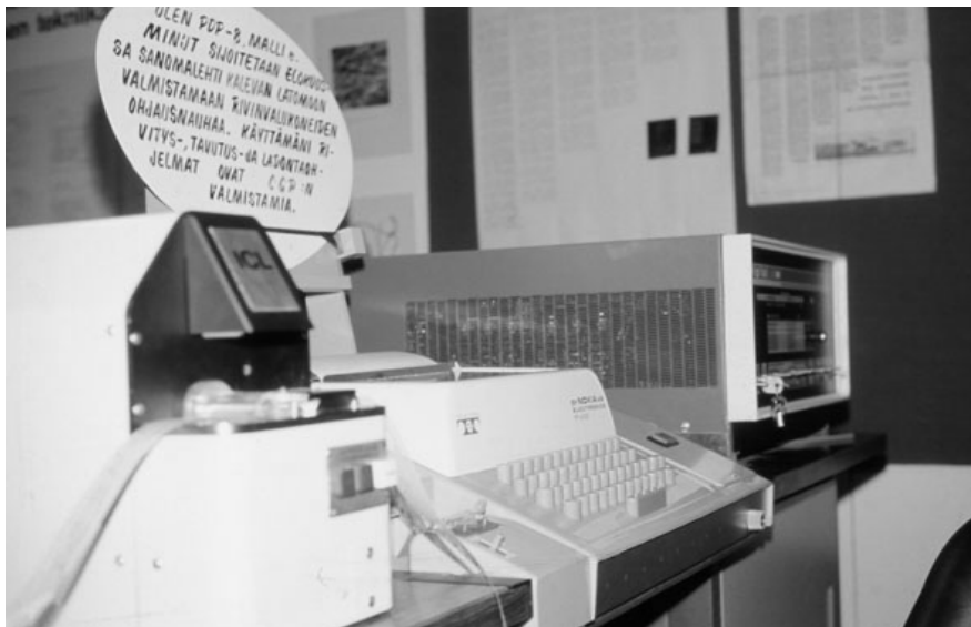
Figure 3: The PDP-8/e based hyphenation and justification system at Kaleva .
