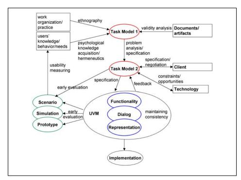
Fig. 5. The DUTCH design method
