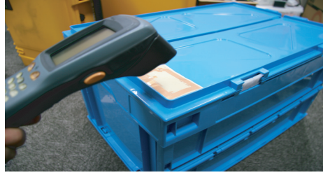
Fig. 8. RFID tag reader scans route specification from tag
