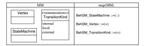
**map(AG):** As mentioned in the mapping from meta-models to abstract grammars, concrete classes and *concatenations* both represent language elements of the model. Therefore, concatenations of the abstract grammar are mapped to concrete classes in the meta-model. The name of the concrete class is derived from the production rule (see below).
