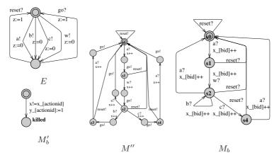
**Fig. 4.** The annotated automata  $(M_a, M_c, M'_a, M'_c, \text{ omitted})$ . The notation v[i] is UppAal notation for indexing array v at position *i*. *bid* is the position for action b
