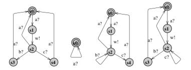
**Fig. 2.** A simple model M and its mutants M[a], M[b], M[c]. The initial location is doubly encircled
