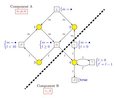
**Fig. 1.** A concurrent machine with two components, which may fail with an unknown severity level and can be repaired accordingly.
