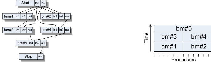
Fig. 1. Example of an M-task application represented by a directed acyclic graph (left) and an appropriate schedule (right). The figure shows the parameter dependencies resulting in a multigraph. The final M-task dag can be derived by combining multiple edges between a pair of nodes into a single edge.
