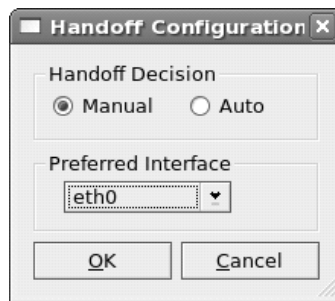
Fig. 7. User of a mobile device can use this graphic interface to choose manual or automatic handover and to assign preferred interface.
