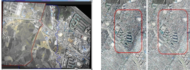
Fig. 7. Mosaic processing using road-based seamlines (a) matching result in urban area (b)
