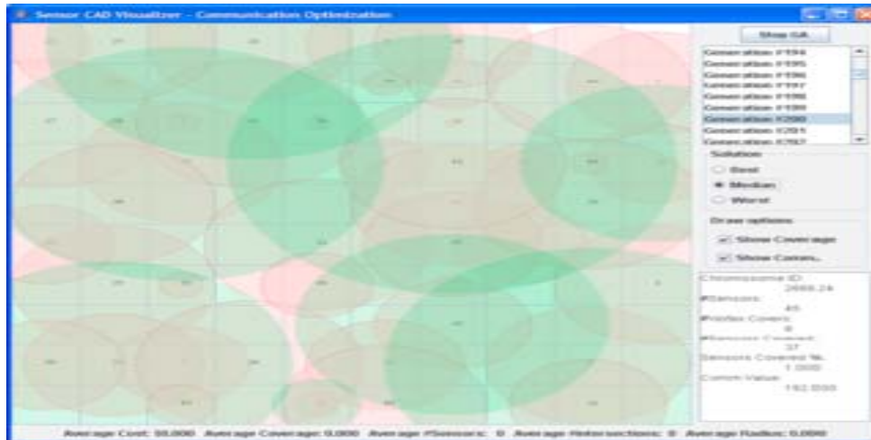
Fig. 9. A snapshot of the Sensor CAD Visualizer, which shows that after 200 generations of applying the communication GA found 8 sensors as the best vertex-cover sensors that cover all coverage sensors.
