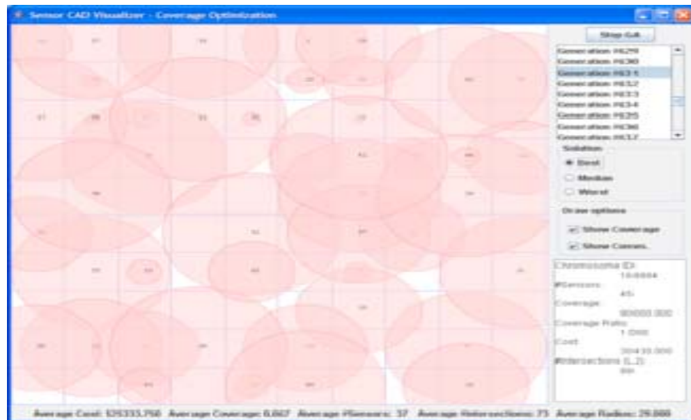
Fig. 8. A snapshot of the Sensor CAD Visualizer, which shows that after 631 generations of applying the coverage GA found 45 sensors as the best coverage at a cost of $30,430 while having a coverage ratio is equal to 99%.
