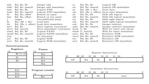
Fig. 1. Instruction set, Programmer's Model, and Instruction Encoding
