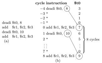
Fig. 2. (a) A code fragment with two *deadline* instructions and (b) its temporal behavior. The *deadline* instruction guarantees the two *add* instructions are executed 8 cycles apart.
