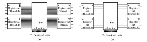
Fig. 5. Reducing the number of register file ports (a) before limiting issue width (b) after limiting issue width to two instructions per thread
