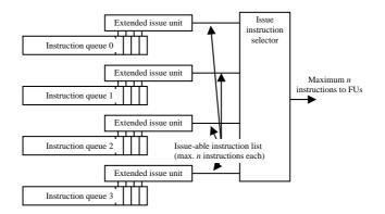
Fig. 2. The Issue Unit of the SMT architecture
