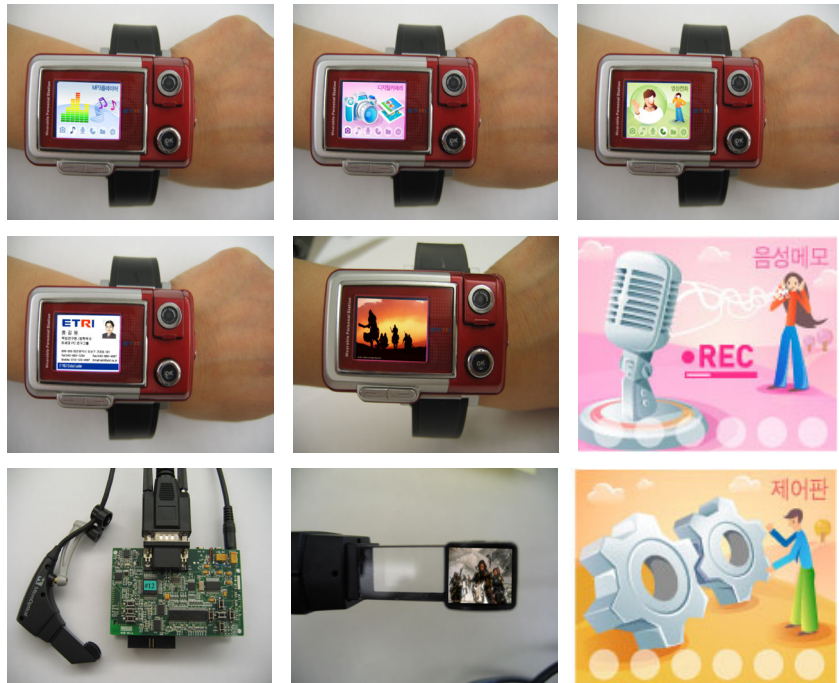
Fig. 6. MP3 Player, Digital Camera, Videophone, Namecard Transfer, MPEG-4 Player, Voice Recorder, Eval B'd with HMD, HMD output and Control Panel
