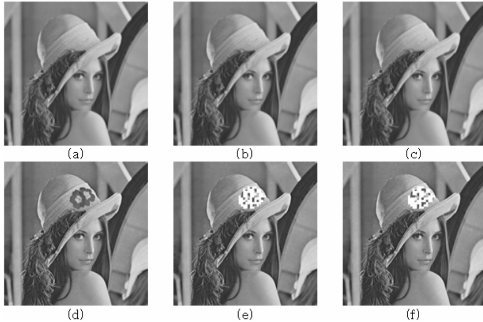
Fig. 2. Detection result of a maliciously manipulated image. (a) is the original image, (b) is the watermarked image (PSNR = 37.8dB), (c) is the JPEG-compressed image (QF = 60%), (d) is the manipulated watermarked image, (e) is the detection result of the manipulated image only, and (f) is the detection result of the JPEG-compressed image (QF = 60%) after manipulation.
