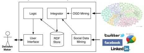
Fig. 3. The Web data oriented architecture
