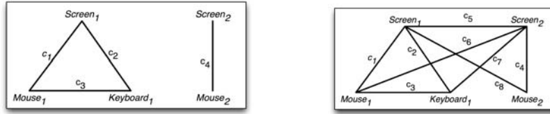
Fig. 4. Left image: the initial configuration that represents a private workstation. Right image: final configuration that corresponds to a public configuration where couplings c_6 , c_7 and c_8 are the consequents of the causal coupling c_5 .
