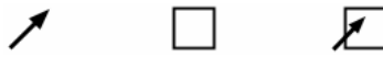
Fig. 1. The three basic symbols underlying the symbolic notation of Canonical Abstract Prototypes (from left to right): a generic abstract tool, a generic abstract material and a generic abstract hybrid, or active material (taken from [2]).
